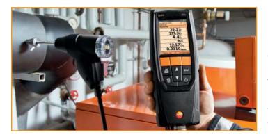
The testo 320 makes your job easier by displaying two to eight user-defined parameters. With eight parameters you see all the measurements simultaneously. No need to scroll up and down chasing the measurements and double guessing.
