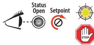
3. Turn the setpoint screw an additional 1/4 turn clockwise for operational margin.
