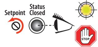
2. Slowly turn the setpoint screw clockwise until the Status OPEN LED just turns ON.
