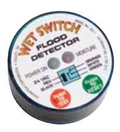
The Wet Switch is a solid state device designed to detect the presence of condensate water overflow. The Wet Switch is placed into the secondary drain pan — a normally dry pan. If the primary drain pan fails, condensate water will overflow into the secondary drain pan. Upon sensing moisture, the Wet Switch will turn the system off (typically the cause of the condensing water) to help prevent damage to carpets, walls, woodwork, ceilings, and other property.
