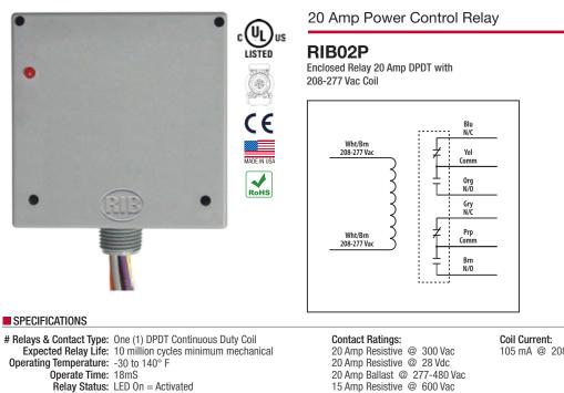
Dimensions: 4.00" x 4.00" x 1.80" with .50" NPT Nipple Wires: 16", 600V Rated Approvals: UL Listed, UL916, UL864, C-UL California State Fire Marshal, CE, RoHS Housing Rating: Plenum, NEMA 1 Gold Flash: Yes Override Switch: No
